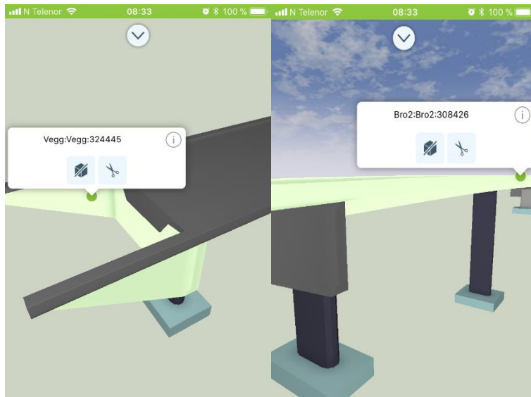
Figure 7–26 An element (abutment) marked in Dalux Field. To mark smaller parts of a bigger component, the component would have to be modeled as several smaller elements or somehow cut into smaller parts. This cannot be done in Dalux Field.
