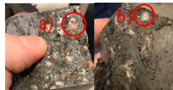
Figure 2: a) breaking in ITZ b) breaking in aggregate
